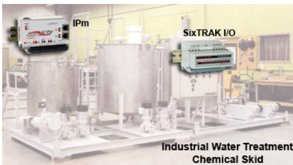
Figure 3 Industrial Water Treatment Application – with Ethernet based micro-controllers and I/Os
