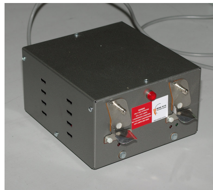
Dual Radio Receiver Integrated Miners Safety Cap Lamp Charger
