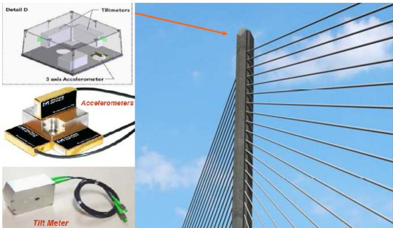
Figure 3 Monitoring Tilts & Vibrations in Piers and Abutments
