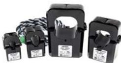
A split-core sensor is used to record AC amperage, for use with the data logger with an input of AC current, sine wave, single phase 50 Hz or 60 Hz, load power factor 0.5 to 1.0 lead or lag. Senses power induced from line voltage using self-gripping split-core design for faster installation. These are available in 5 ranges - 20, 50, 100, 200 & 600 Amps. This is used to estimate electrical draw on the motors. We use the runtime data to estimate actual kilowatt hour usage for each motor.
