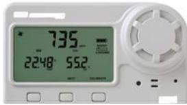
Indoor CO<sub>2</sub>, RH and Temperature logger makes it more convenient than ever to measure and record CO<sub>2</sub> in buildings and other non-condensing environments. It measures CO<sub>2</sub> from 0–5,000 parts per million (ppm).
