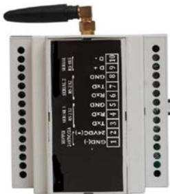
The IoT gateway is a Microcontroller based product with GSM interface for connecting field instruments with cloud. It collects real time data from field instruments and pushes data to cloud server. Data stored at cloud server can be viewed from remote places. The gateway stores data in local non-volatile flash memory in case of network issue and sends data to the server when network connection is restored to avoid data loss. It supports MQTT Protocol.
